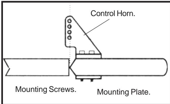
3) Position the rudder control horn on the left side of the airplane. Mount the control horn parallel with the horizontal stabilizer.
