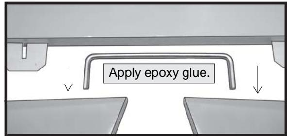
Glue the elevator hinges in place using the same techniques used to hinge the ailerons.
