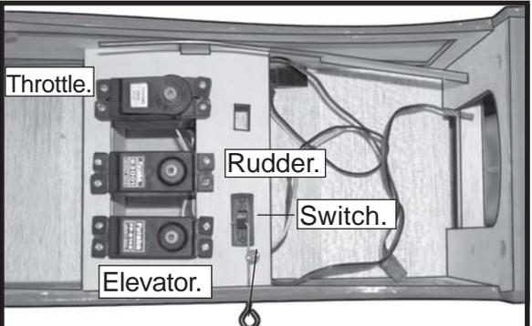
5) Install adjustable servo connector in the servo arm.
