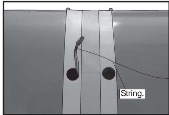
5) Tape the servo lead to the wing to prevent it from falling back into the wing.
