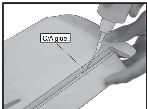
5) Turn the wing panel over and deflect the aileron in the opposite direction from the opposite side. Apply thin C/A glue to each hinge, making sure that the C/A penetrates into both the aileron and wing panel.
