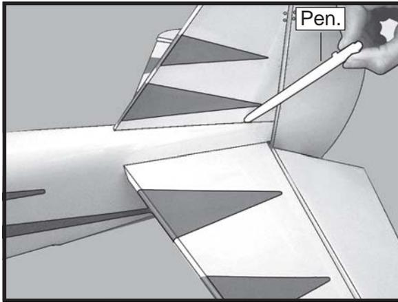
4) Remove the stabilizer. Using the lines you just drew as a guide, carefully remove the covering from between them using a modeling knife.
