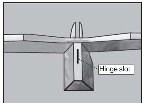
2) Slide the vertical stabilizer into the slot in the top of the fuselage. The rear edge of the stabilizer should be flush with the rear edge of the fuselage and the lower rudder hinge should engage the precut hinge slot in the lower fuselage. The bottom edge of the stabilizer should also be firmly pushed against the top of the horizontal stabilizer.
