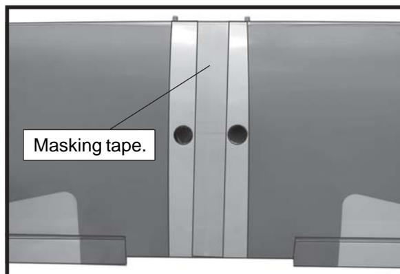
3) When the epoxy has cured, carefully remove the masking tape from the wing.
