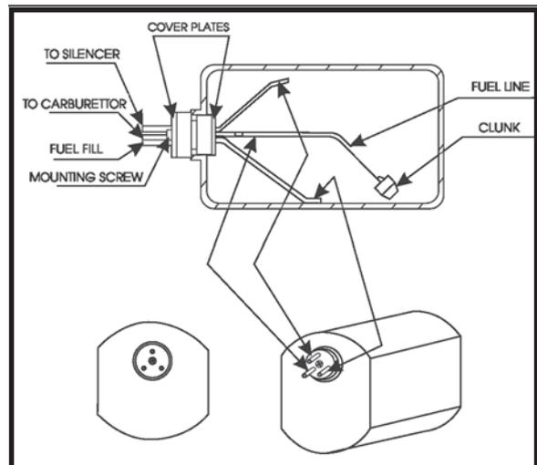
Attach the silicone fuel and pressure pipes to the tank. The lower pipe is the 'feed' and the upper two the 'pressure and fill'. The fill pipe is the next pipe.
