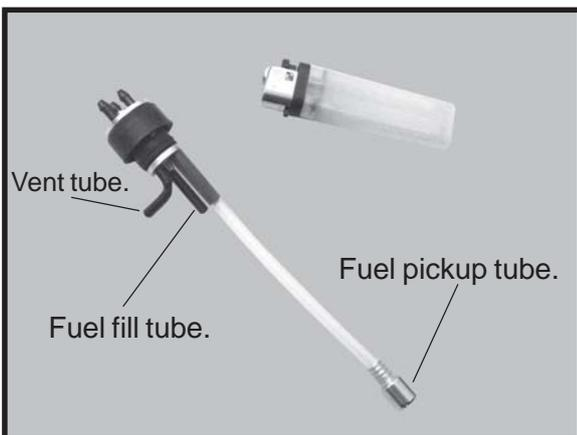
**Important:** *When the stopper assembly is installed in the tank, the top of the vent tube should rest just below the top surface of the tank. It should not touch the top of the tank.*
