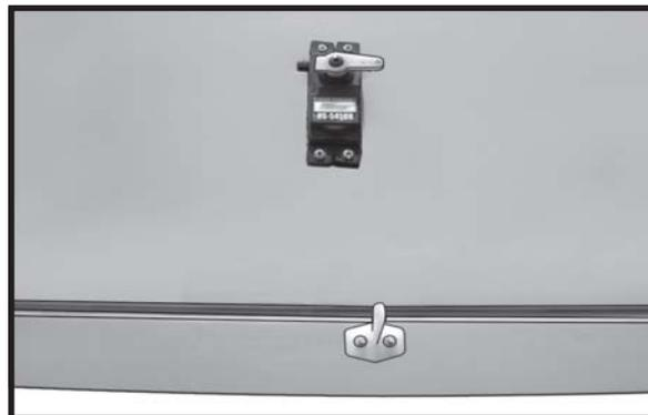
6) Thread one nylon adjustable control horn onto each aileron control rod. Thread the horns on until they are flush with the ends of the control rods.
