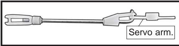
9) Connect the linkage as shown and secure the control wire with a wire keeper.
