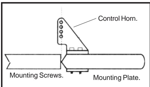
4) Using a 1mm drill bit and the control horns as a guide, drill the mounting holes through the aileron halves.
