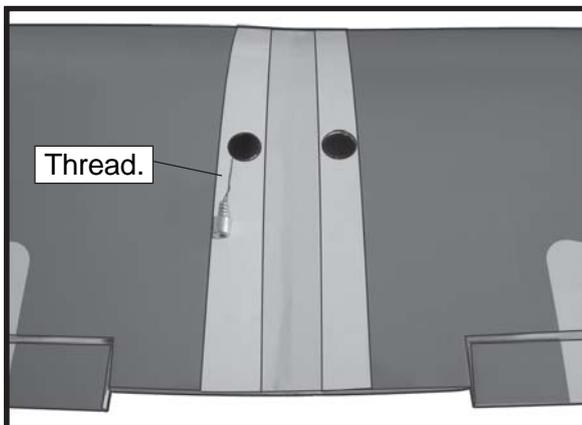
4) Attach servo lead to the aileron servo. Attach the string to the servo lead and carefully thread it through the wing. Once you have thread the lead through the wing, remove the thread so it can use for the other servo lead.
