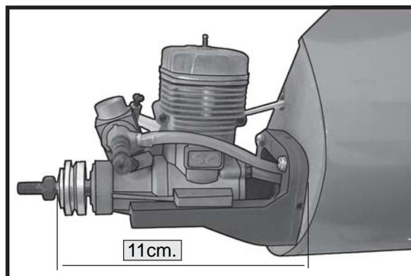
2) Place your engine onto the engine mount. Adjust the engine is centered of the edges of the engine case.
