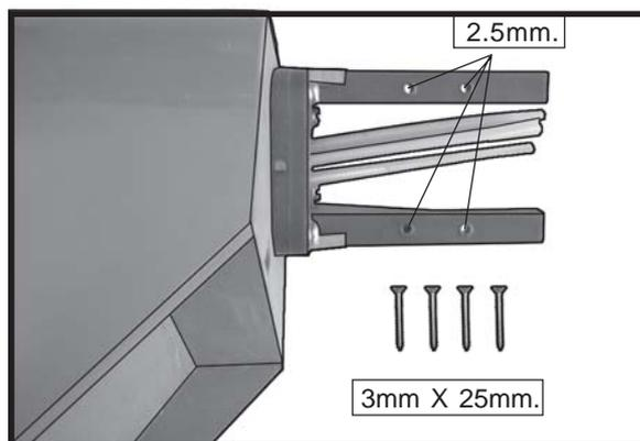
5) Bolt the engine to the engine mount using the four machine screws. Double check that all the screws are tight before proceeding.
