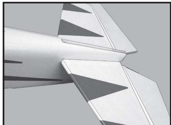
3) With the stabilizer held firmly in place, use a pen and draw lines onto the stabilizer where it and the fuselage sides meet. Do this on both the right and left sides and top and bottom of the stabilizer.
