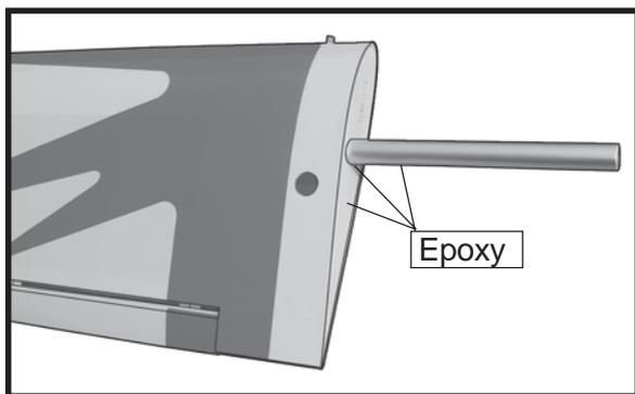
Carefully slide the two wing halves together and firmly press them together, allowing the excess epoxy to run out. There should not be any gap in the wing halves. Use rubbing alcohol and a paper towel to clean up any excess epoxy.
