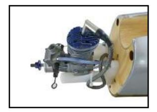
Blow through one of the lines to ensure the fuel lines have not become kinked inside the fuel tank compartment. Air should flow through easily.
