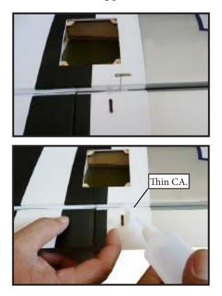
5) Turn the wing panel over and deflect the aileron in the opposite direction from the opposite side. Apply thin C/A glue to each hinge, making sure that the C/A penetrates into both the aileron and wing panel.
