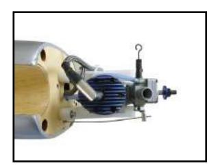
8) Connect the Z-bend in the 450mm throttle pushrod to the outer hole of the thottle servo arm.
