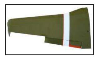
Note : Work the flap up and down several times to "work in" the hinges and check for proper movement.
