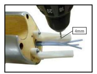
4) On the fire wall has the location for the throttle pusshrod tube (pre-drill).
