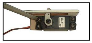
6) Apply 1-2 drops of thin C/A to each of the mounting tabs. Allow the C/A to cure without using accelerator.
