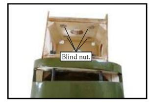
5) Attach the motor to the front of the electric motor box using four 4mm blind nut, four M3x15mm hex head bolts to secure the motor. Please see picture shown.
