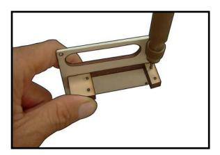
3) Apply 2-3 drops of thin C/A to each of the mounting holes. Allow the C/A to cure without using accelerator.
