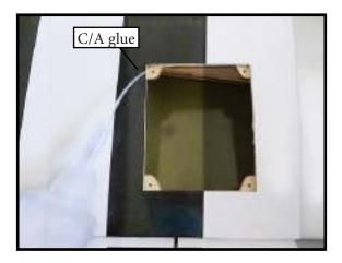
7) Remove the string from the wing at the servo location and use the tape to attach it to the servo extension lead. Pull the lead through the wing and remove
