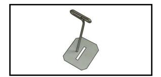
2) Remove each hinge from the wing panel and aileron and place a T-pin in the center of each hinge. Slide each hinge into the wing panel until the T-pin is snug against the wing panel. This will help ensure an equal amount of hinge is on either side of the hinge line when the aileron is mounted to the aileron.
