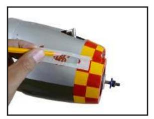
4) Slide the muffler screws through the engine. Place the mufflr extension and gaskets included with the engine on the screws. Be careful when mounting the cowl so the screws and extension remain in position until the mufflr can be attached.
