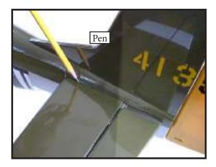
5) Remove the stabilizer. Using the lines you just drew as a guide, carefully remove the covering from between them using a modeling knife. When cutting through the covering to remove it, cut with only enough pressure to only cut through the covering itself. Cutting into the balsa structure may weaken it.
