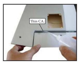
5) Turn the wing panel over and deflect the flap in the opposite direction from the opposite side. Apply thin C/A glue to each hinge, making sure that the C/A penetrates into both the flap and wing panel.
