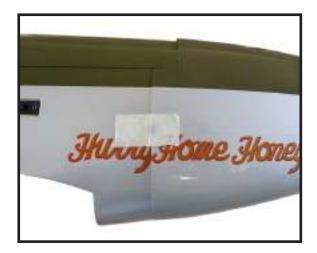
2) Use a drill and drill bit to drill the holes for the cowl mounting screws. Make sure the cowl position is correct before drilling each hole.
