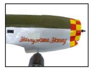
3) Tape a piece of card stock to the fuselage to indicate the location of the mufflr, needle valve, and any other items that may require access when the cowl is mounted. Slide the cowl on the fuselage, and transfer these locations onto the cowl. Use a drill, rotary tool and sanding drum to make any cut-outs in the cowl before securing it to the fuselage.
