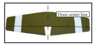
2) Using a modeling knife, carefully remove the covering at mounting slot of horizontal stabilizer ( both side of fuselage).
