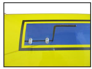
Be careful not to overtighten the set screws. Overtightening may cause the threads to strip.
