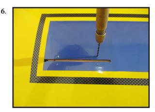
Remove the two straps and the gear wire. Drill four 3/32" pilot holes into the wing for the wood screws.
