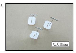
Remove each hinge from the wing panel and aileron and place a T-pin in the center of each hinge. Slide each hinge into the wing panel until the T-pin is snug against the wing panel. This will help ensure an equal amount of hinge is on either side of the hinge line when the aileron is mounted to the aileron.
