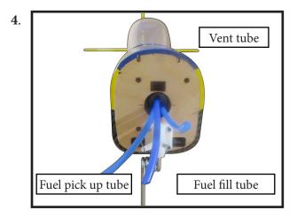
Connect the lines from the tank to the engine and muffler. The vent line will connect to the muffler and the line from the clunk tothe carburetor.
