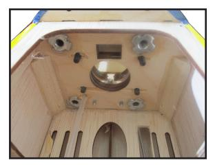
Attach the motor mount to the front of the electric motor box using four 4mm blind nut, four M4x25mm hex head bolts to secure the motor. Please see picture shown.
