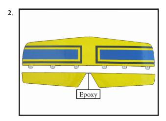
Glue the elevator hinges in place using the same techniques used to hing the ailerons.
