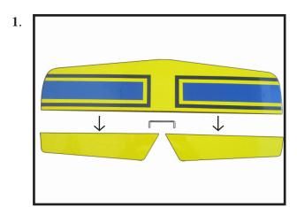
Carefully remove the elevator from one of the horizontal stabilizer panels. Note the position of the hinges.
