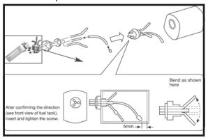
☐ 5. Test fit the stopper assembly into the tank. It may be necessary to remove some of the flashing around the tank opening using a modeling knife. If flashing is present, make sure none of it falls into the tank.
