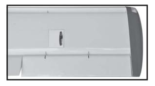
$\Box$  5. Instal servo tray with aileron servo into the wing as same as picture below.
