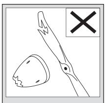
NEVER use damaged or deformed propellers or spinners.
