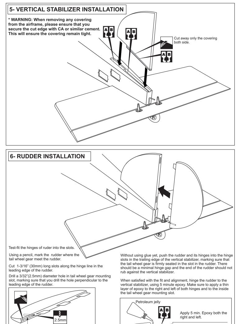
Tail wheel gear mounting slot
