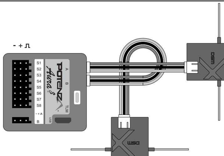
Note: It may be necessary to move the ESC lead to another open port (such as 'Port B') during the binding procedure. Be sure to return the ESC lead back to S1 after binding is complete.
