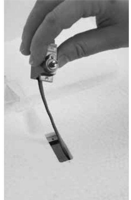
**TIP:** Plug a spare servo extension into the servo lead before removing to make it easier to install the lead of the servo when replaced.
