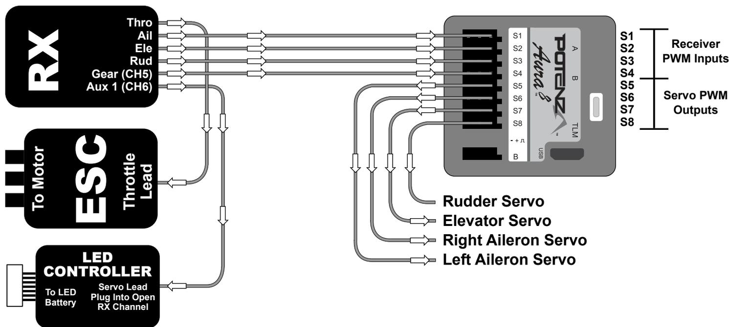
Note: The LEDs on the QQ Extra 300G2 Night Version are able to be turned on and off via a channel from your transmitter. For PWM users, simply plug the servo lead from the LED controller into any open channel on your receiver (such as CH6/AUX1), and assign that channel to a 2-position switch on your transmitter accordingly.
