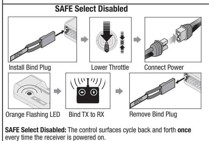
SAFE Select can also be activated via Forward Programming in compatible transmitters.
