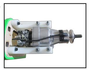
I Thread nylon tie through mounting holes.
