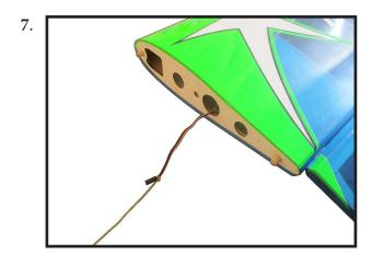
Tape the servo lead to the wing to prevent it from falling back into the wing.
