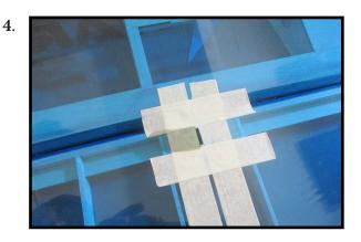
Remove the control horns from the control surfaces. Apply epoxy to the slot in the aileron and flap. Make sure the epoxy gets into the slot for a good bond between the surfaces and control horn.
