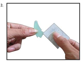
Check the fit of the control horns to the aileron and flap. They should rest flush against the control surface as shown.
