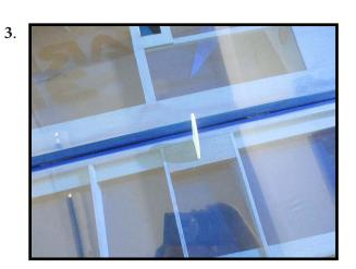
Place low-tack tape 1/32 inch (1mm) from the control horn slot. This will prevent epoxy from getting on the control surface when the control horns are glued in place.
