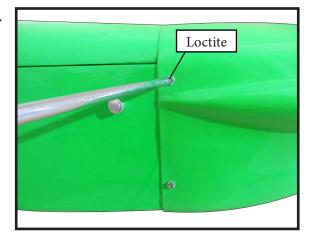
Install the muffler and muffler extension onto the engine and make the cutout in the cowl for muffler clearance. Connect the fuel and pressure lines to the carburetor, muffler and fuel filer valve. Secure the cowl to fuselage using the M3x10mm socket head screws.Putting a small length of silicon fuel tube under the head of the screw helps with
